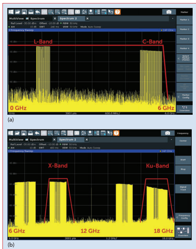
▲ Fig. 8 EV12DD700 simultaneous output: L- and C-Bands (a), X- and Ku-Bands (b).
